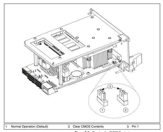
Figure 2-3. Clearing the CMOS Contents
